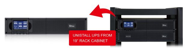
After UPS is uninstalled from 19" rack cabinet, UPS unit will be available to service center for repair. Individual PDU module stays on 19" rack cabinet will keep supplying AC power to loadings without interruption.
